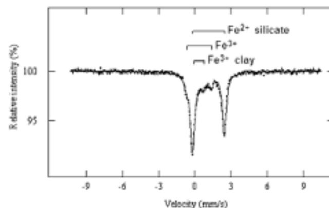
**Figure 3.** Mössbauer spectrum of GC1806 with 5000 y B.P. at 77K. Parameters of specific  $\text{Fe}^{3+}$  are IS of  $0.55 \pm 0.01$  and QS of  $1.79 \pm 0.02\text{ mm s}^{-1}$ .
