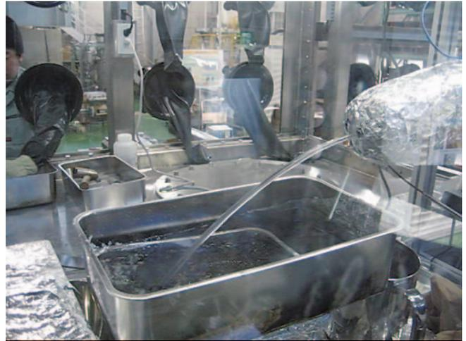
**Figure 2.** Photo of discharged molten LiCl-KCl salt flow from freeze-seal valve.
