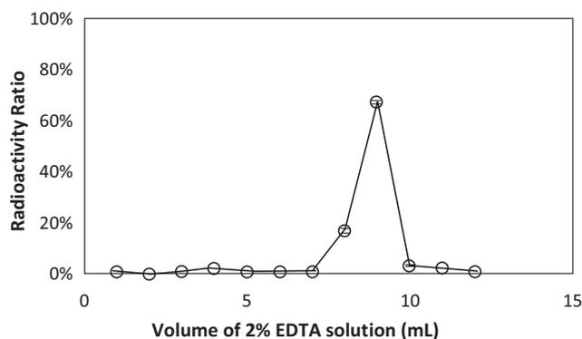
**Figure 3.** Elution curve of  $^{89}\text{Sr}$  from the cation-exchange column by 3.25 M HCl. The elution profile was determined using 2 mL aliquots. The y-axis is the activity ratio of eluted  $^{89}\text{Sr}$  to initially added  $^{89}\text{Sr}$ .
