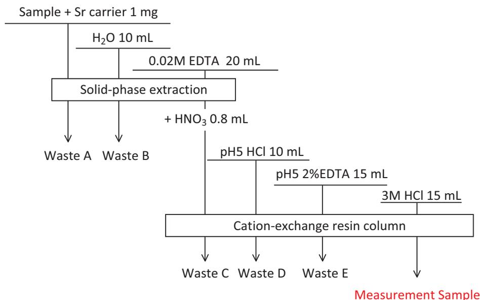
**Figure 1.** Schematic of the chemical separation procedure for the isolation of <sup>90</sup>Sr from aerosol samples by solid-phase extraction
