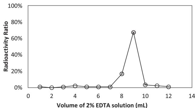
**Figure 2.** Elution curve of  $^{210}\text{Pb}$  from the cation-exchange column by 2% EDTA solution at pH = 5. The elution profile was determined using 1 mL aliquots. The y-axis is the activity ratio of eluted  $^{210}\text{Pb}$  to initially added  $^{210}\text{Pb}$ .
