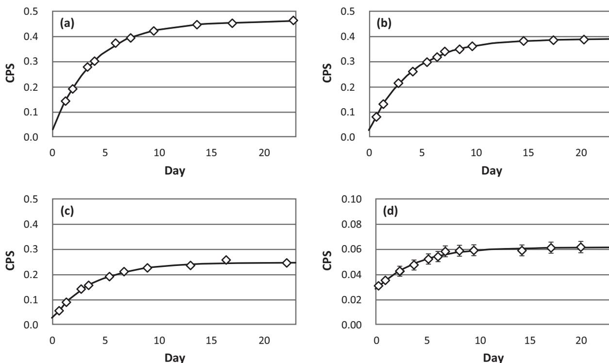
**Figure 4.** Yttrium-90 growth curves from  $^{90}\text{Sr}$  in (a) MIT4, (b) MIT9, (c) MIT12, and (d) MIT13 aerosol samples. The data points were obtained by the 1220 QUANTULUS™ counter. The solid lines are the  $^{90}\text{Y}$  growth, calculated by fitting the counting data to the equation for radioactive equilibrium.
