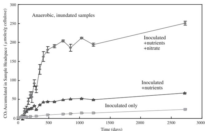
**Figure 3.**  $\text{CO}_2$  production in anaerobic, brine-inundated cellulose samples. The accumulation of  $\text{CO}_2$  in each set of samples displays two distinct gas generation phases: a rapid increase in the first 500 days followed by a long period of slow accumulation.
