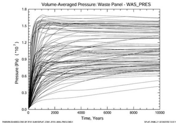
**Figure 4.** Evolution of Disposal Room Pressure in the WIPP Repository. The pressure buildup in the repository is partly due to microbial degradation of organic materials in the wastes.
