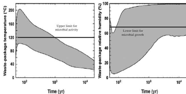
**Figure 2.** Thermal and Relative Humidity Histories Predicted for YM Repository and Their Constraints on Microbial Growth (modified from BSC, 2004).<sup>38</sup>
