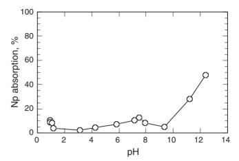
Figure 1. Adsorption of Np(V) on bentonite over a wide range of pHs under aerobic conditions.
