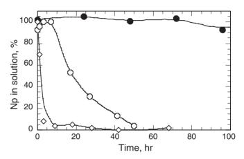
**Figure 2.** Microbial mediated removal of Np(V). Removal of Np by bentonite under aerobic conditions ( $\bullet$ ), with 0.01 mol/L Na<sub>2</sub>S ( $\bigcirc$ ) and with cells ( $\Box$ ). Conditions: bentonite, 0.5 g/L; NaNO<sub>3</sub>, 0.01 mol/L; Np, 1 × 10<sup>-6</sup> mol/L.
