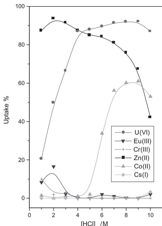
**Figure 16.** Sorption of U(VI), Eu(III), Cr(III), Zn(II), Co(II), and Cs(I) from HCl solutions by TDA-impregnated resin,  $[\text{TDA}]_{(r)} = 0.96$  mol/kg.
