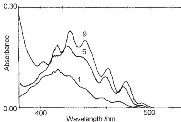
**Figure 6a.** Absorption spectra of aqueous uranyl chloride solutions (0.015 M) in the presence of HCl acid at different concentrations; numerals on curves are initial aqueous HCl concentrations (M).
