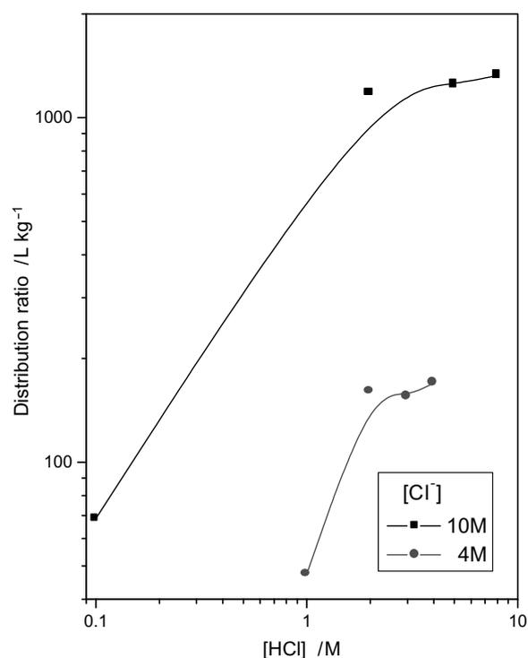
**Figure 3.** Effect of HCl concentration on sorption of U(VI) at constant chloride ion concentration;  $[\text{TDA}]_{(r)} = 1.05$  mol/kg-sorbent.
