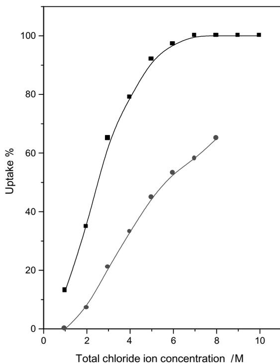
**Figure 2.** Extraction of U(VI) from HCl and LiCl solutions by TDA-impregnated resin (■: in presence of HCl only, ●: in presence of 0.1 M HCl and LiCl),  $[\text{TDA}]_{(r)} = 0.96$  mol/kg-sorbent.
