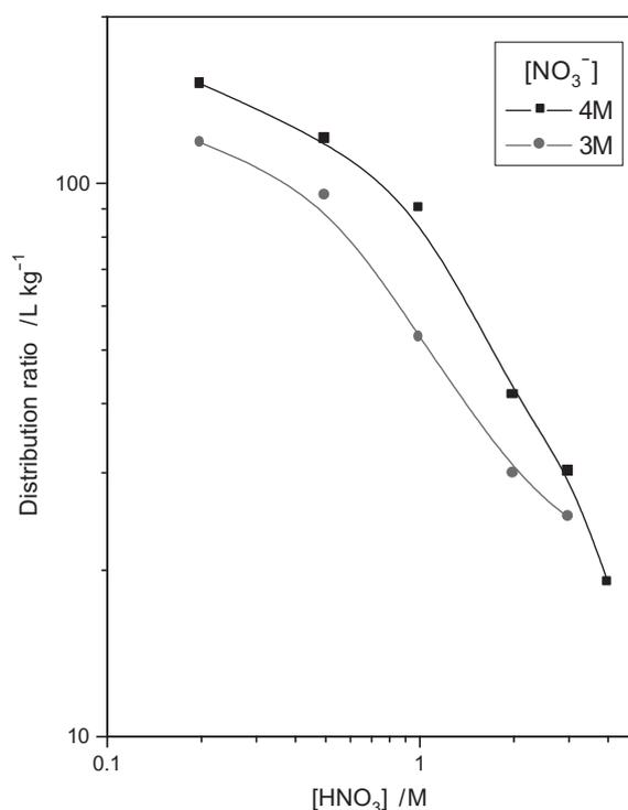
**Figure 12.** Effect of HNO<sub>3</sub> concentration on distribution of Th(IV) at constant nitrate ion concentration; [TDA]<sub>(r)</sub> = 0.96 mol/kg.
