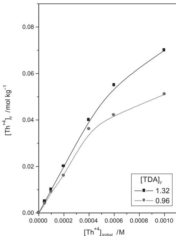
**Figure 14.** Effect of initial aqueous  $Th^{4+}$  concentration on amount of  $Th^{4+}$  sorbed from 0.2 M  $HNO_3$  + 5.8 M  $LiNO_3$  solution with TDA-impregnated resin;  $[TDA]_{(r)}$  in the unit of mol/kg.
