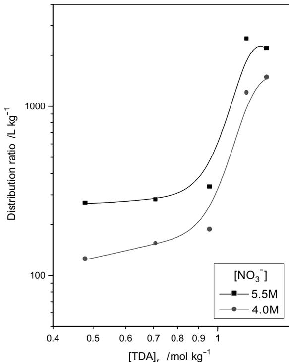
**Figure 13.** Effect of TDA concentration on extraction of Th(IV) from nitrate media (0.2 M  $HNO_3$  +  $LiNO_3$ ).
