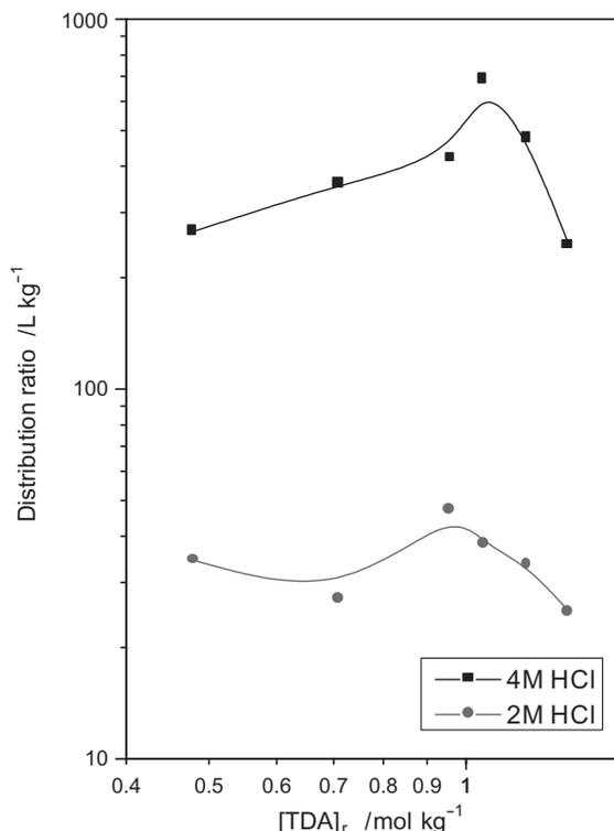
**Figure 4.** Effect of TDA concentration on extraction of U(VI) from HCl solutions.
