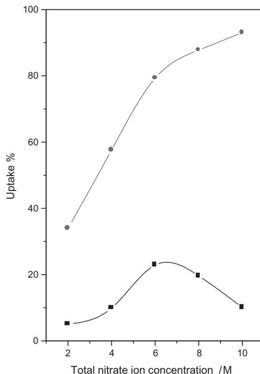
**Figure 11.** Extraction of Th(IV) from HNO<sub>3</sub> and LiNO<sub>3</sub> solutions by TDA-impregnated resin (■: in presence of 0.2 M HNO<sub>3</sub> and LiNO<sub>3</sub>, ●: in presence of HNO<sub>3</sub> only); [TDA]<sub>(r)</sub> = 0.96 mol/kg.
