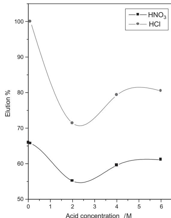
**Figure 15.** Effect of HCl or  $HNO_3$  concentration on elution of Th(IV) loaded on TDA-impregnated resin;  $[Th^{4+}]_{(r,initial)} = 5 \times 10^{-3}$  mol/kg,  $m = 0.05$  g,  $V = 5$  mL,  $[TDA]_{(r)} = 0.96$  mol/kg.
