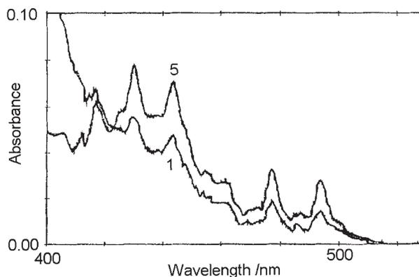
**Figure 6b.** Absorption spectra of benzene solutions of uranium species extracted at different HCl concentrations; numerals on curves are initial aqueous HCl concentrations (M),  $[\text{TDA}]_{(r)} = 1.05 \text{ mol/kg}$ .
