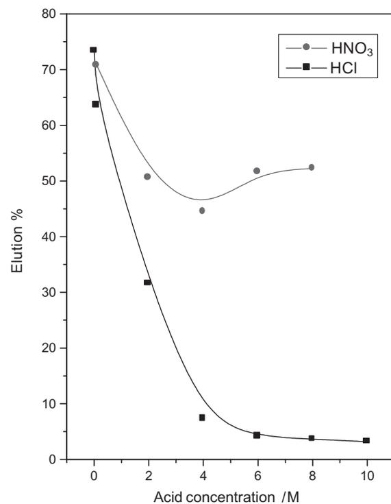
**Figure 9.** Effect of  $\text{HCl}$  or  $\text{HNO}_3$  concentration on elution of U(VI) loaded on TDA-impregnated resin;  $[\text{U}]_{(r, \text{initial})} = 0.008$  mol/kg,  $m = 0.05$  g,  $V = 5$  mL,  $[\text{TDA}]_0 = 0.96$  mol/kg.
