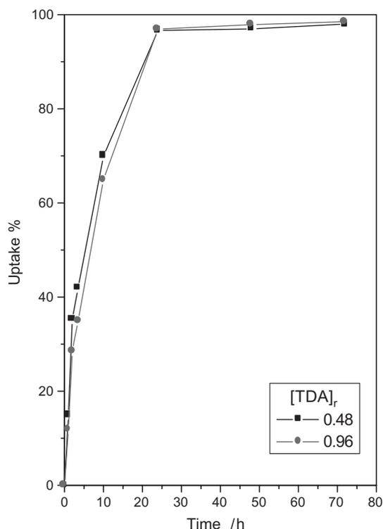
**Figure 10.** Effect of contact time on sorption of Th(IV) from 6 M nitrate solution (0.2 M HNO<sub>3</sub> + 5.8 M LiNO<sub>3</sub>) with TDA-impregnated resin; [TDA]<sub>(r)</sub> in the unit of mol/kg.
