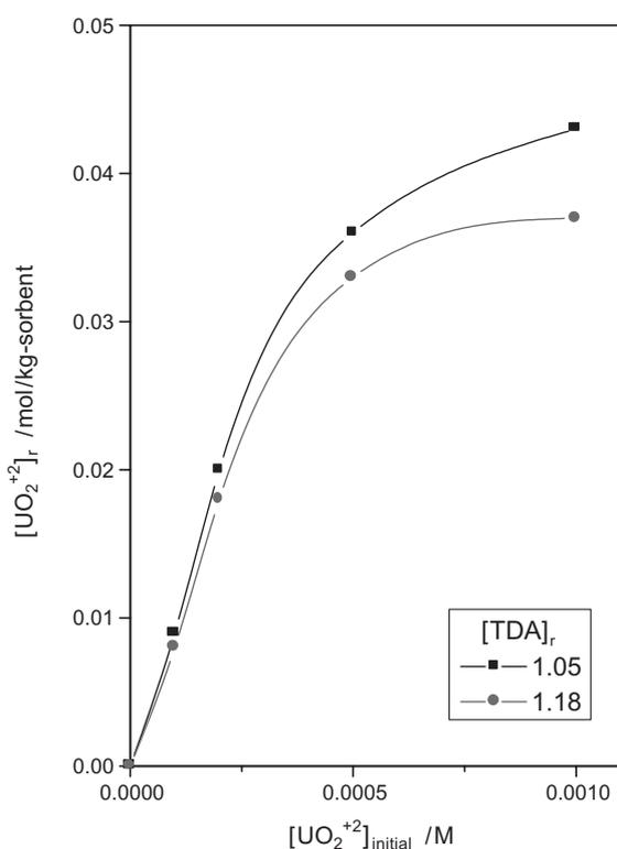
**Figure 5.** Effect of initial aqueous  $\text{UO}_2^{2+}$  concentration on amount of  $\text{UO}_2^{2+}$  sorbed from HCl solution by TDA-impregnated resin;  $[\text{HCl}] = 7 \text{ M}$ ,  $[\text{TDA}]_{(r)}$  in the unit of mol/kg-sorbent.
