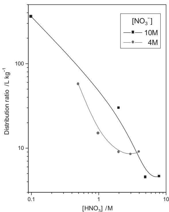
**Figure 8.** Effect of  $\text{HNO}_3$  concentration on sorption of U(VI) at constant nitrate ion concentration;  $[\text{TDA}]_0 = 1.05$  mol/kg-sorbent.
