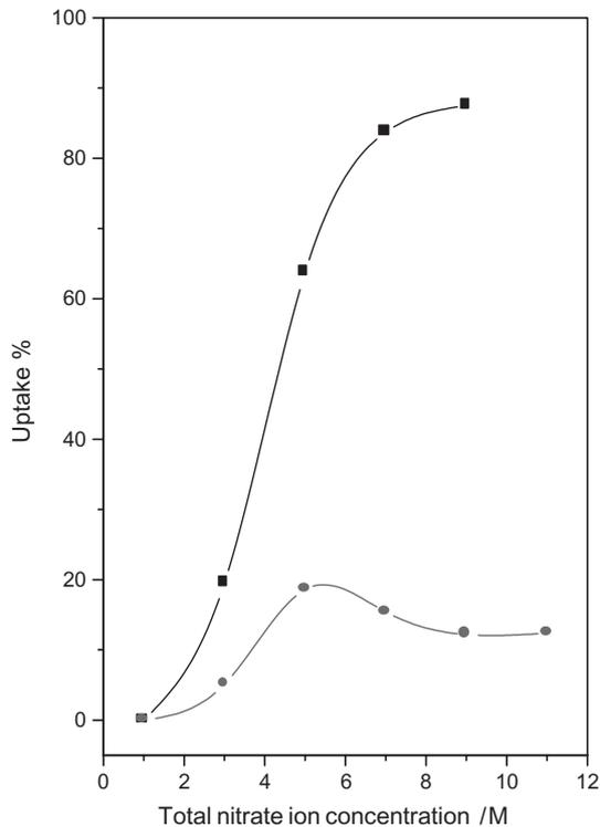
**Figure 7.** Extraction of U(VI) from  $\text{HNO}_3$  and  $\text{LiNO}_3$  solutions by TDA-impregnated resin (■: in presence of 0.2 M  $\text{HNO}_3$  and  $\text{LiNO}_3$ , ●: in presence of  $\text{HNO}_3$  only),  $[\text{TDA}]_0 = 0.96$  mol/kg-sorbent.
