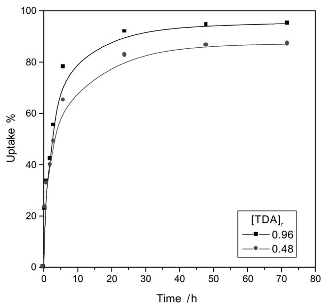
**Figure 1.** Effect of contact time on sorption of U(VI) from 6 M HCl with TDA-impregnated resin;  $[\text{TDA}]_{(r)}$ : in the unit of mol/kg.
