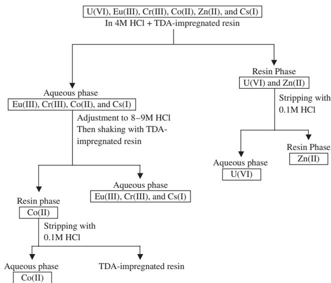
**Figure 17.** Flowsheet diagram for separation of U(VI), Eu(III), Cr(III), Co(II), Zn(II), and Cs(I).
