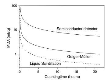
Figure 3. Taken from Reference 64. Minimum Detectable Activities for different detectors as a function of the counting time.
