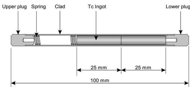
**Figure 1.** ANTICORP 1 pin drawings.
