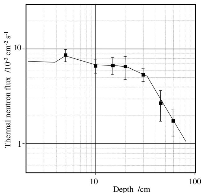
**Figure 2.** Depth profile of thermal neutron flux in soil.
