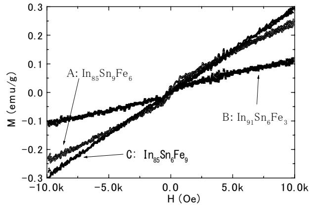
Fig1 Magnetization of Fe doped ITO
