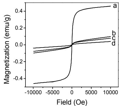
Fig.1 Magnetization curves for samples: a)  $\text{Sn}_{0.85}\text{Sb}_{0.05}\text{Fe}_{0.1}\text{O}_{2-\delta}$ , b)  $\text{Sn}_{0.8}\text{Sb}_{0.1}\text{Fe}_{0.1}\text{O}_{2-\delta}$ , c)  $\text{Sn}_{0.9}\text{Fe}_{0.1}\text{O}_{2-\delta}$ , d)  $\text{Sn}_{0.85}\text{Sb}_{0.1}\text{Fe}_{0.05}\text{O}_{2-\delta}$ .
