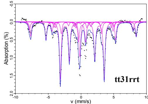
図1 Mössbauer spectrum of nanowires produced in CNTs. (at room temperature, tt28rrt) 図2 Mössbauer spectrum of nanowires produced in CNTs. (at room temperature, tt31rrt)
