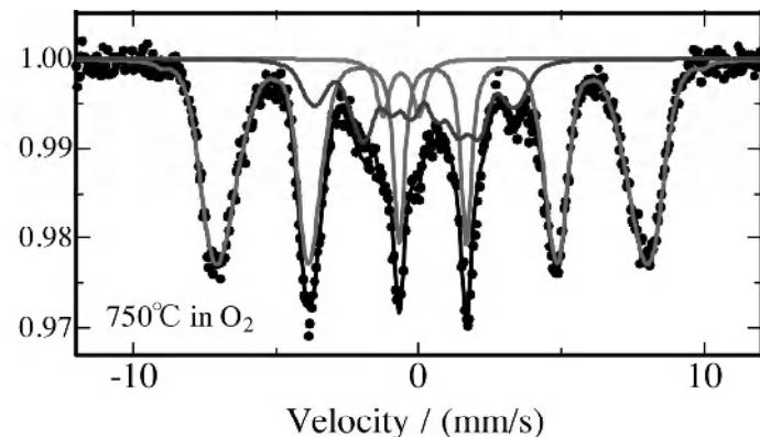
Fig. 1 Mössbauer spectrum at 5 K of 30% Fe-doped  $\text{Li}_2\text{MnO}_3$  annealed at 750°C in  $\text{O}_2$ .
