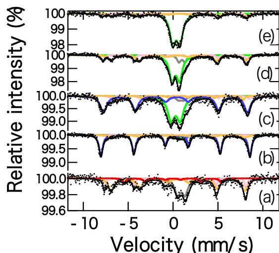
Fig.1 Mössbauer spectra of the films produced by laser deposition of  $\text{Fe}_2\text{O}_3$  in  $\text{O}_2$  atmosphere. (a) In vacuum, and the  $\text{O}_2$  pressures are (b)7Pa (c)45Pa (d)120Pa, and (e)200Pa..
