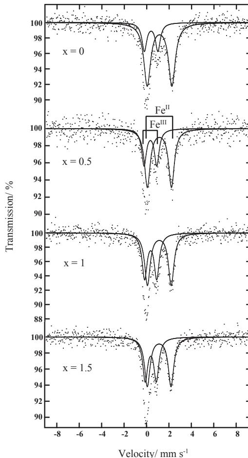
Fig.1. Mössbauer spectra of xLi<sub>2</sub>O-2FeO-V<sub>2</sub>O<sub>5</sub>-P<sub>2</sub>O<sub>5</sub> (x=0, 0.5, 1, and 1.5) glasses measured at room temperature.
