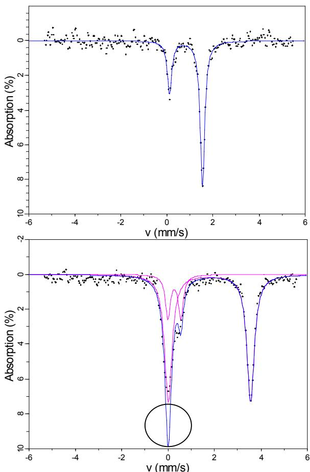
FIG.1. Mössbauer spectra taken with a source Rh( $^{57}\text{Co}$ ) and  $\text{FePSe}_3$  single crystal absorber at room temperature (upper) and 30K (lower).
