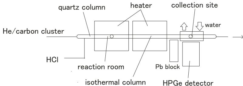
Fig.1 Schematic diagram of experimental apparatus
