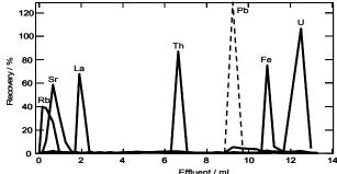
Fig.1 Chromatogram of the representative elements with a pressurized anion-exchange system.
