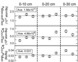
Fig.1 Comparison of ratios among fallout nuclides,  $^{239+240}$ Pu/ $^{137}$ Cs,  $^{236}$ U/ $^{137}$ Cs and  $^{236}$ U/ $^{239+240}$ Pu in the soil cores form Ishikawa pref. Japan.
