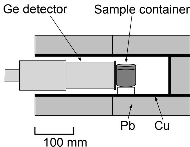
**Figure 3.** Schematic drawing of our detector setup for measurements of soil samples.
