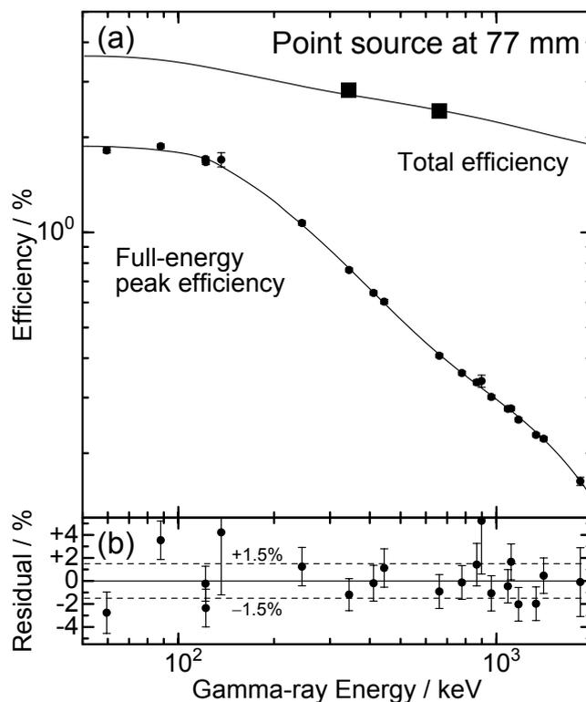
**Figure 1.** (a) Total and full-energy peak efficiencies for point sources placed at a source-to-detector distance of 77 mm. (b) Residuals of the measured full-energy peak efficiency values to the fitted curve.
