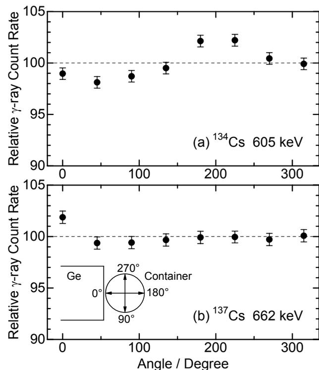
**Figure 4.** Relative  $\gamma$ -ray count rates observed at 8 different directions of the sample container for (a)  $^{134}\text{Cs}$  and (b)  $^{137}\text{Cs}$  in the standard soil samples. The geometry of the detector and the sample container is also drawn in the figure.
