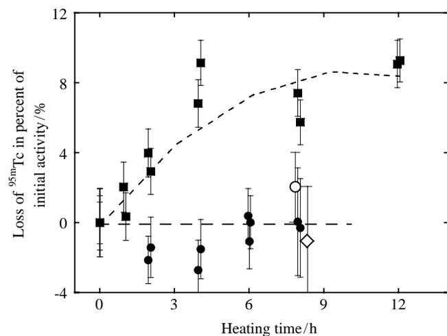
**Figure 1.** Loss of  $^{95m}\text{Tc}$  from soil samples as a function of heating time when incinerated at  $450^\circ\text{C}$ . Freshly contaminated soil (○); 1-month contaminated Andosol (□); 1-month contaminated Gray lowland soil (△); 6-month contaminated soil (◇). Bars indicated counting errors.
