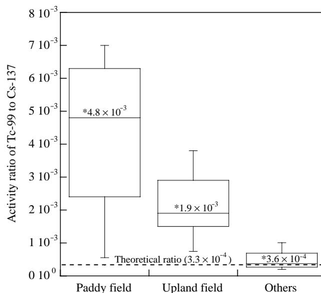
**Figure 5.** Activity ratios of  $^{99}\text{Tc}$  to  $^{137}\text{Cs}$  in soil samples collected in Japan. \*: geometric mean
