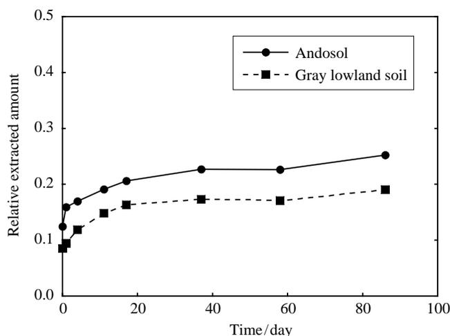
**Figure 8.** Time dependence on the amounts of CA-extractable Tc in the air-dried Andosol and GLS following waterlogging. The soil samples were waterlogged for 52 days then air-dried for 86 days. Each extraction was carried out in duplicate.
