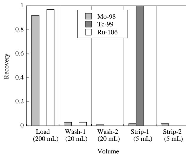
**Figure 3.** Recoveries of  $^{99}\text{Tc}$ , Ru and Mo in load (0.1M  $\text{HNO}_3$ ), wash (2M  $\text{HNO}_3$ ) and strip (8M  $\text{HNO}_3$ ) solutions. The sample solutions were pure water.
