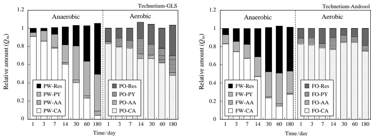
**Figure 7.** Time dependence on the amounts of CA-, AA- and PY-extractable Tc in GLS and Andosol under waterlogged and upland field water conditions. PW: GLS under waterlogged conditions, PO: GLS under upland field conditions, FW: Andosol under waterlogged conditions and FO: Andosol under upland field conditions. CA, AA, PY and Res are explained in Table 3.
