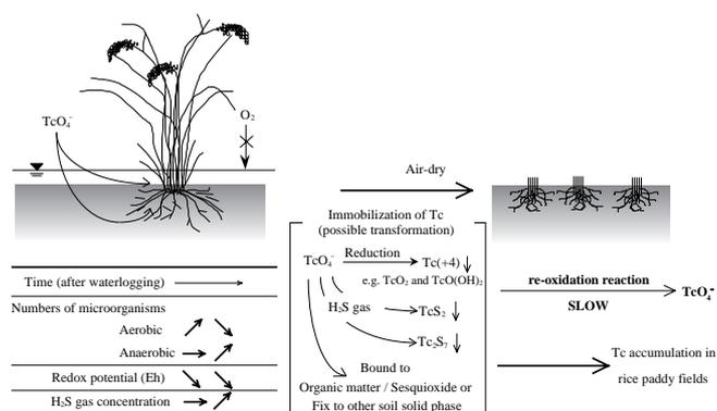
**Figure 9.** Immobilization mechanism of Tc in paddy field soil.
