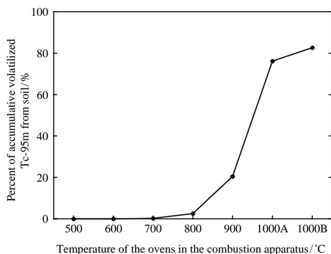
**Figure 2.** Temperature effect on Tc volatilization from a soil sample. The soil sample was volatilized for 1 h at each temperature. 1000A and 1000B: First and second volatilizations at  $1000^\circ\text{C}$ .
